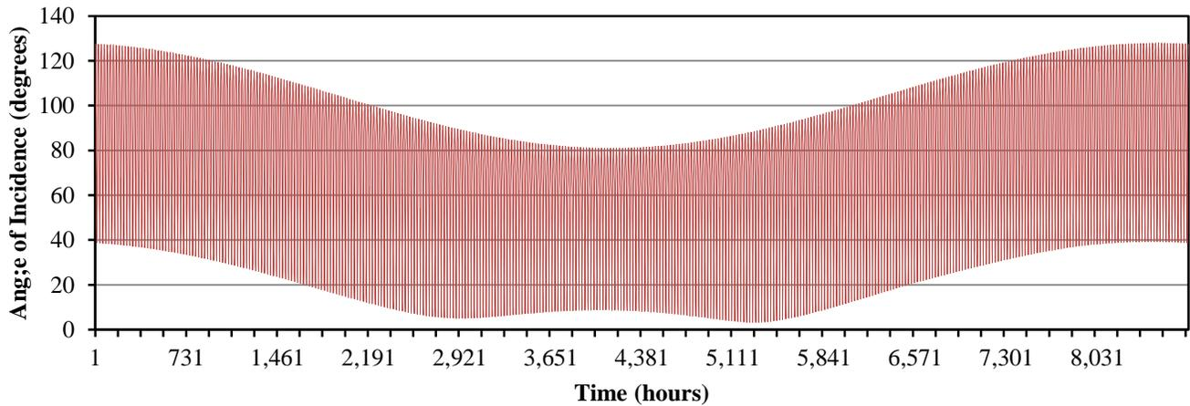
The incident angle is the angle between the line normal to the irradiated surface and the earth-sun line. It affects the direct component of the solar radiation striking the surface and the ability of the surface to absorb, transmit or reflect solar irradiation.
