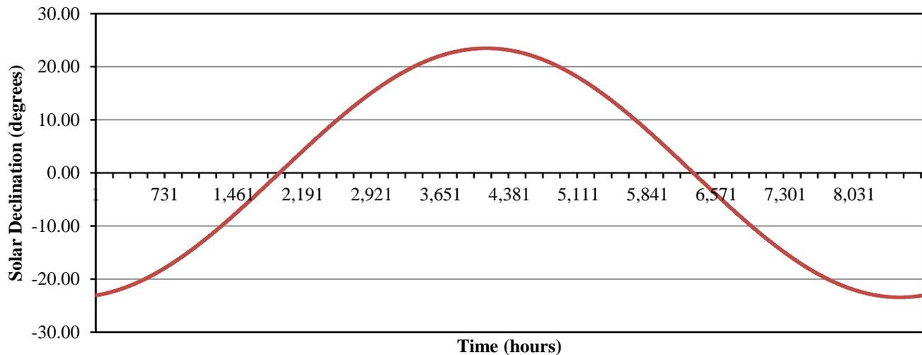
Solar declination is the angle between the earth-sun line and the earth's equatorial plane. This angle varies with date and can be approximated using the following equations. The change in solar declination is the primary reason for our changing seasons.
