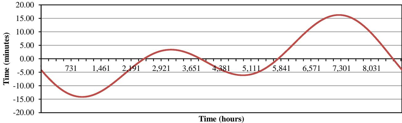
The equation of time represents the difference between apparent solar time (AST) and mean solar time (MST) for a given location due to obliquity of the ecliptic and the eccentricity of earth's orbit around the sun. It varies over the course of a year according to the following expression:
